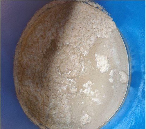
20 mins Settling for sludge formation
